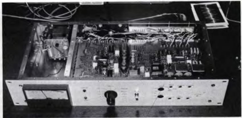
Here you see inside. Note in the upper right corner that the input connections are shielded inside the unit.
